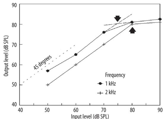
**Figure 2.** Input–output curves at 1 kHz and 2 kHz obtained from probe-tube microphone measurements in the ear canal of a patient with a DACS device. The arrows indicate the level of device saturation.
