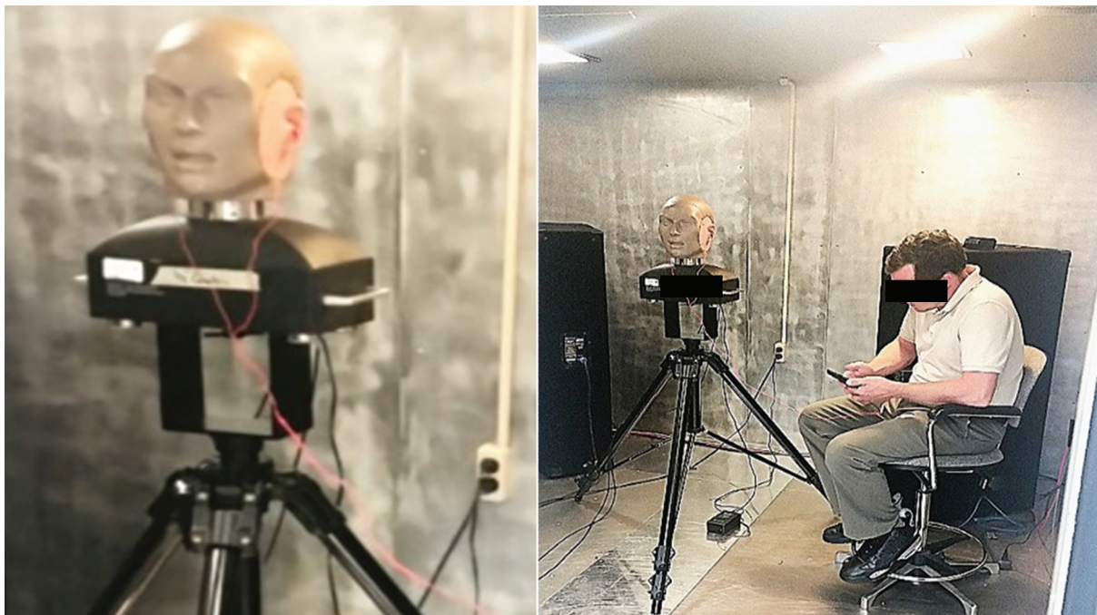
Figure 2. GRAS 45CB acoustic test fixture (ATF) and testing lab setting during data collection
